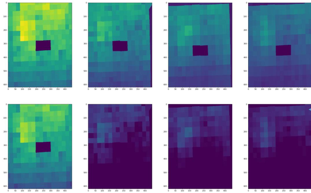
Test deconvolution with (bottom) and without (top) mean background subtraction. Bins of 0.9, 6.9, 8.9, 10.9 MeV
