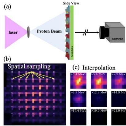
Probies is a high repetition rate pixelated spatial-spectral proton detector
