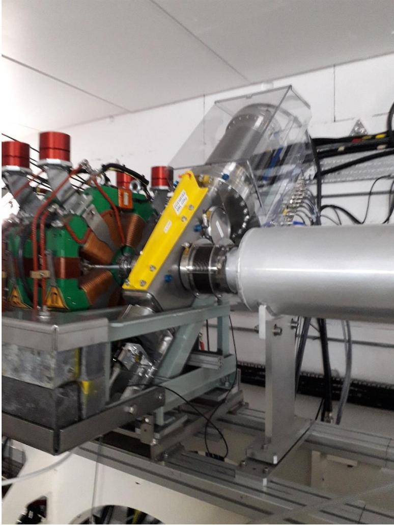
Profile monitor using carbon nanotube wires
