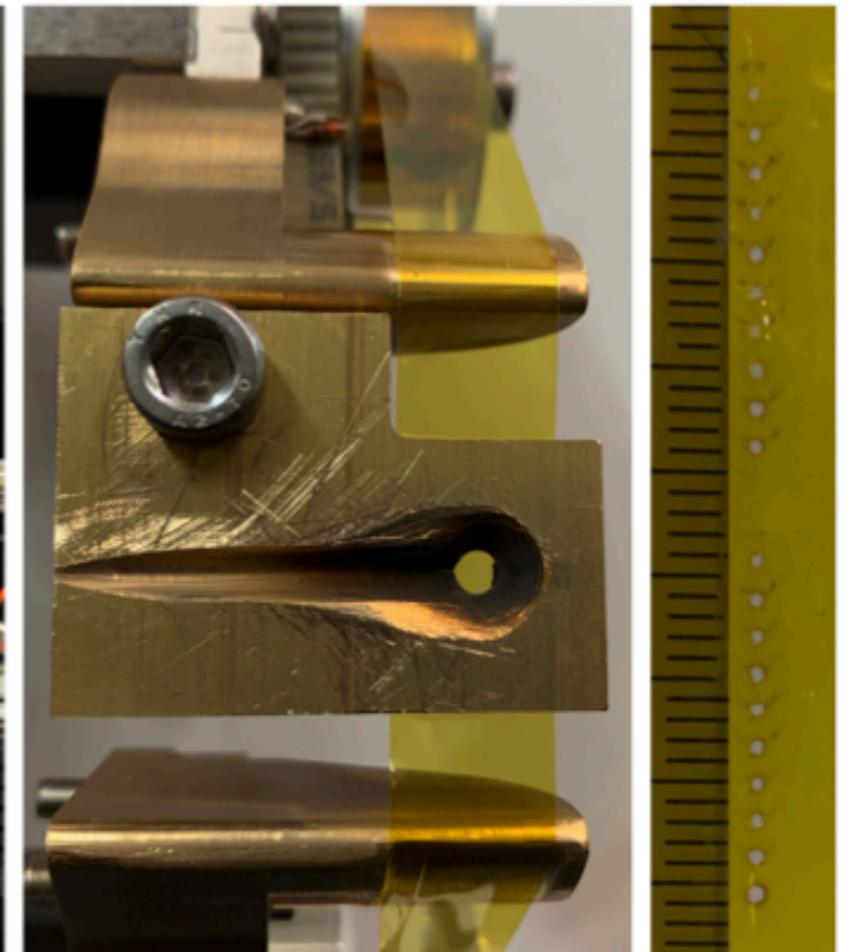
High stability homemade tape target for 100 Hz operation
