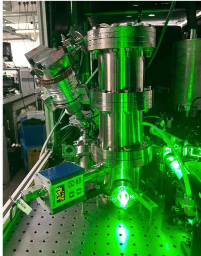
Cryogenic regenerative amplifier and 4-pass amplifier to mitigate thermal lensing
