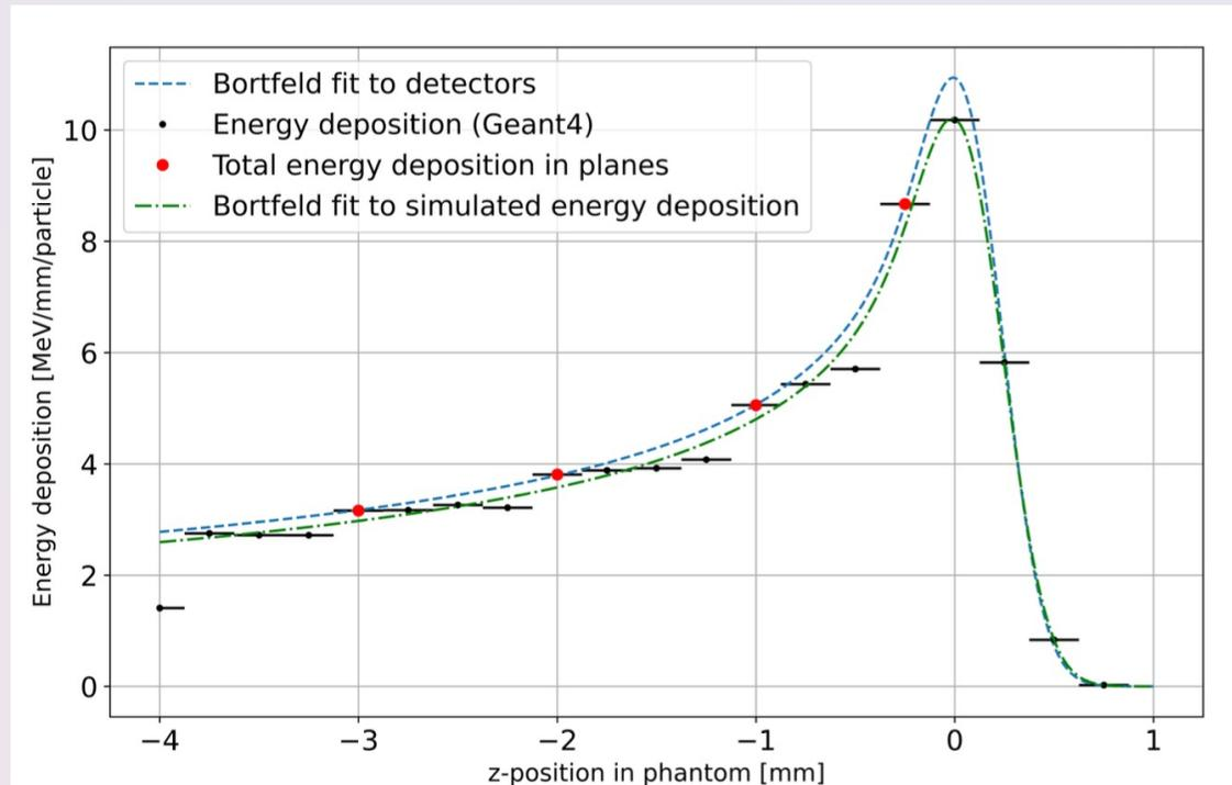
Figure 15: Histogram of the energy deposited by the proton beam in the water phantom as a function of position (taken from Anthea's & Vania's thesis).
