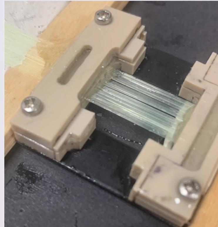
Figure 20: Fibre plane manufacturing (taken from Anthea's & Vania's thesis).
