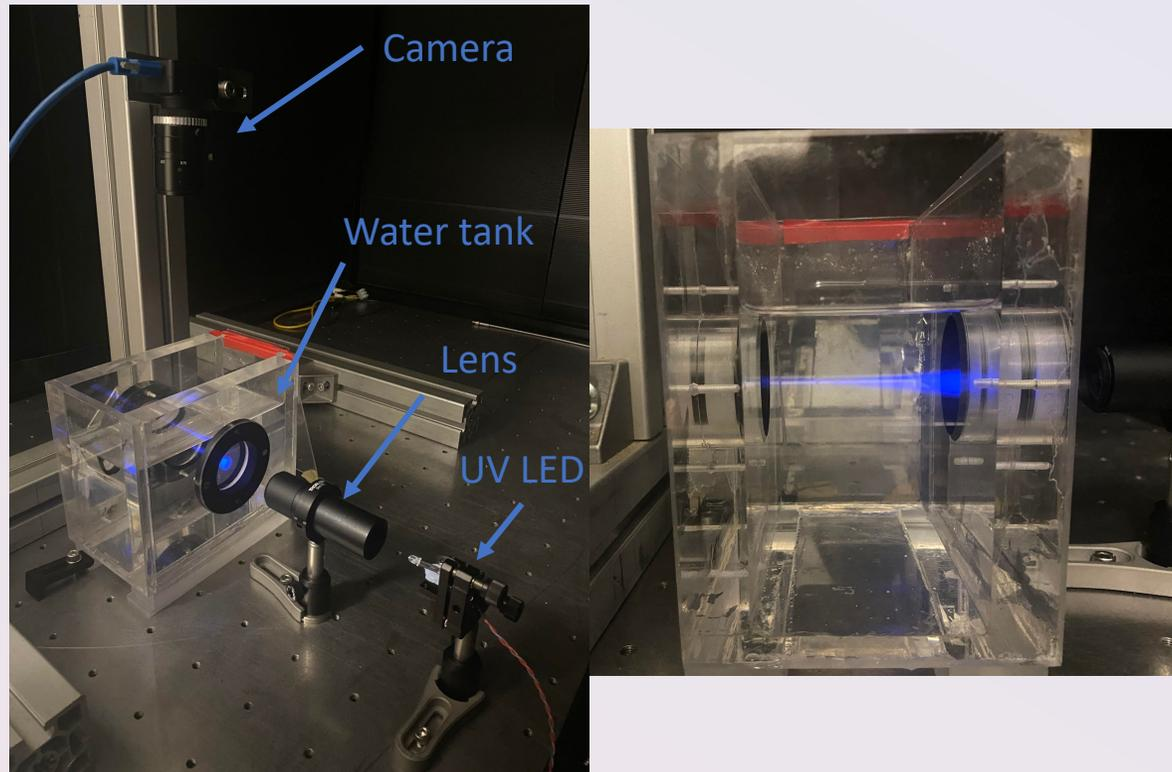
Figure 23: Fluorescent dye experimental set up: angled view (left), cross-section view (right).
