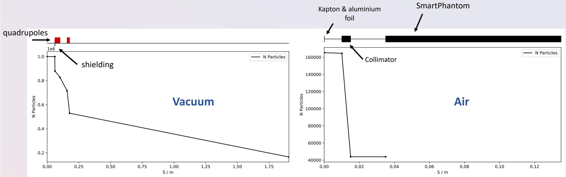
Figure 6: Particle depletion through the vacuum (left) and air (right) section of the simulated beamline.
