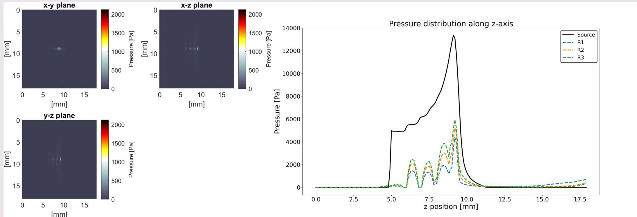
Figure 16: Reconstructed pressure distribution using an iterative time reversal algorithm , with 4 stations of scintillating fibre planes.
