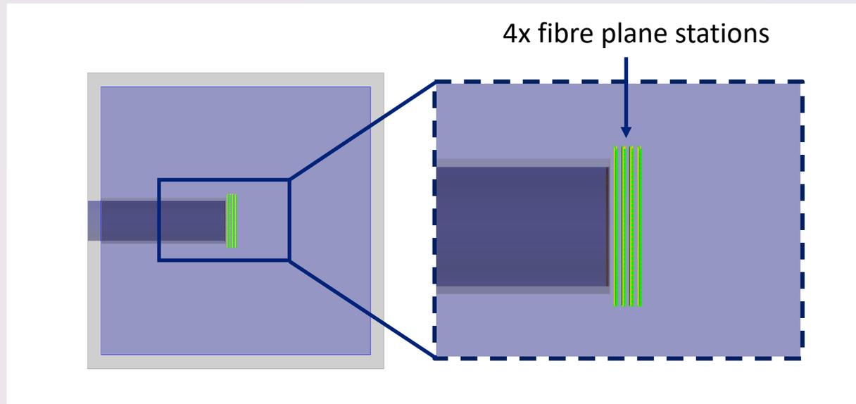
Figure 13: Scintillating fibre plane stations (green) in the Geant4 simulation geometry, Off-axis view (left), side-on view (right).
