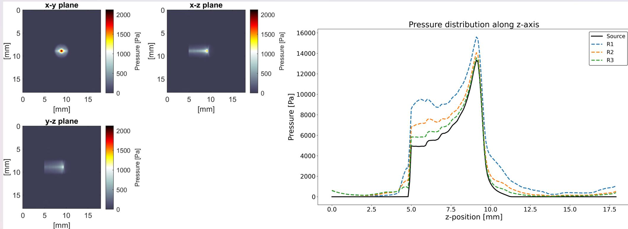
Figure 11: Reconstructed pressure distribution using an iterative time reversal algorithm.
