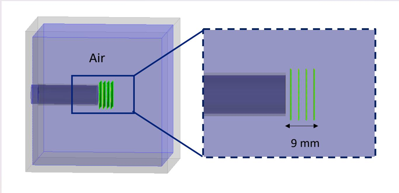
Figure 17: Scintillating fibre plane stations (green) in the Geant4 simulation geometry. Off-axis view (left), side-on view (right).
