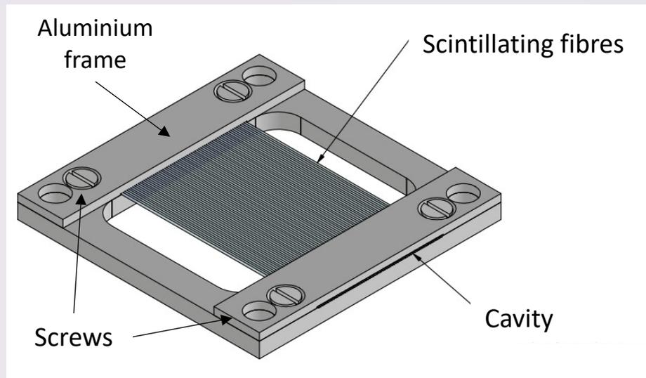
Figure 19: Fibre plane CAD design.
