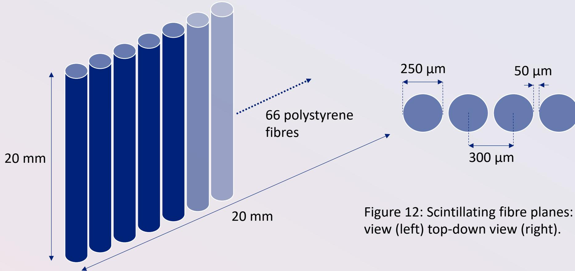
Figure 12: Scintillating fibre planes: off-axis view (left) top-down view (right).
