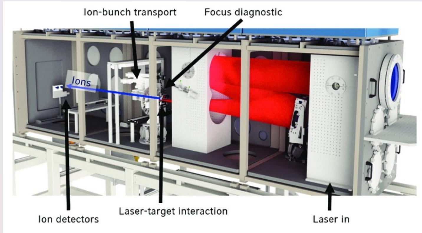
Figure 1: Rendered CAD model of the LION beamline [1].
