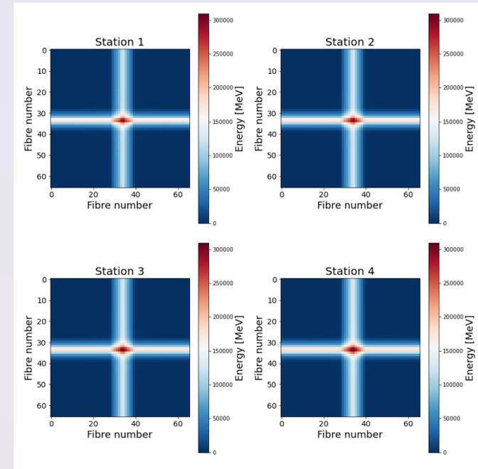
Figure 18: 2D energy distribution reconstruction at each SciFi station.
