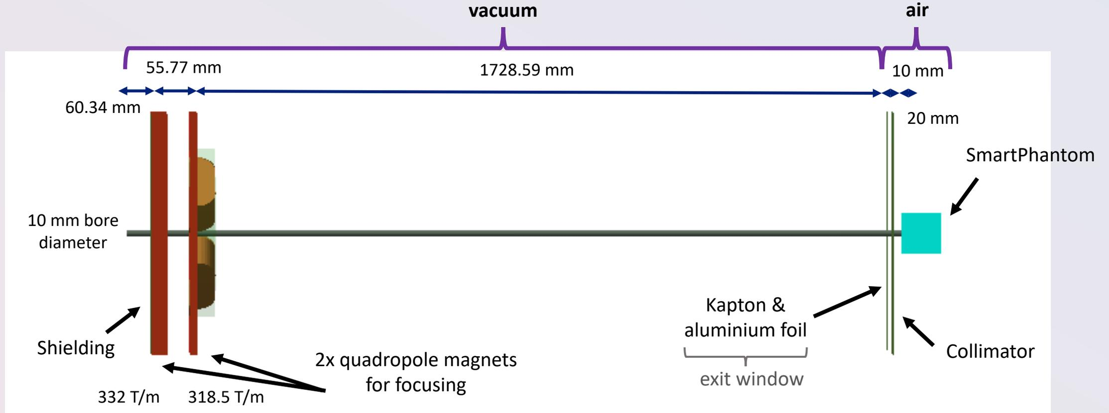
Figure 5: Side-on view of LION beamline in BDSIM.
