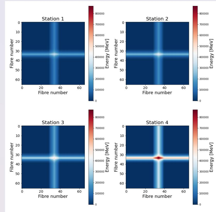
Figure 14: 2D energy distribution reconstruction at each SciFi station.
