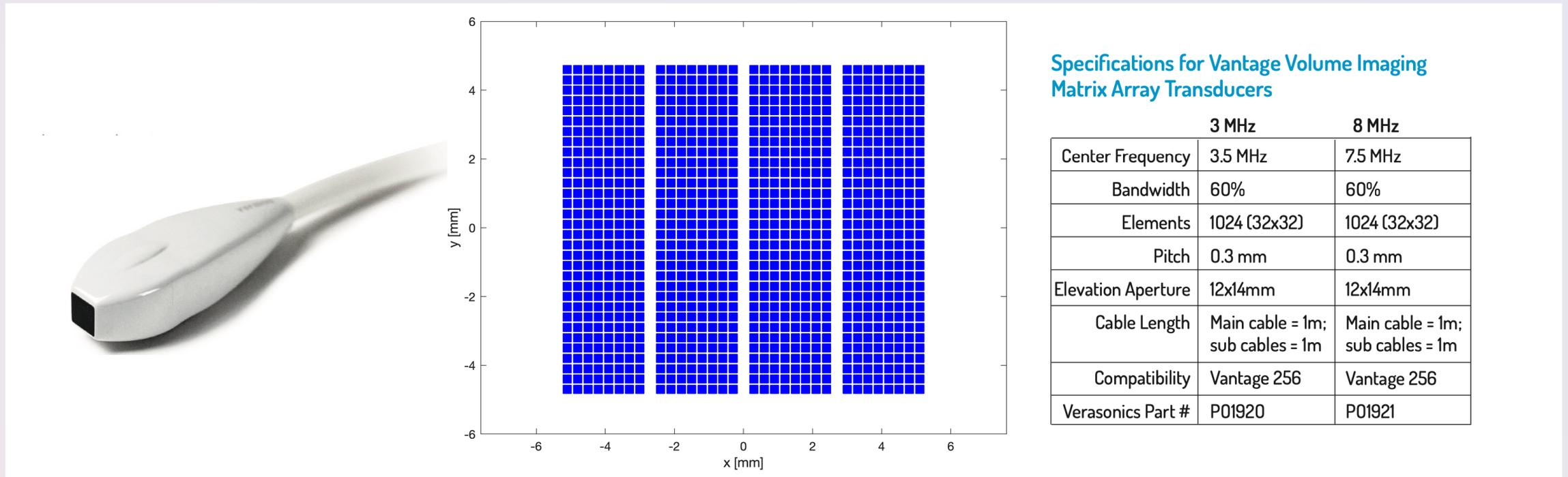
Figure 26: Matrix array shape (left), element configuration (middle) and detailed specifications (right) [3].
