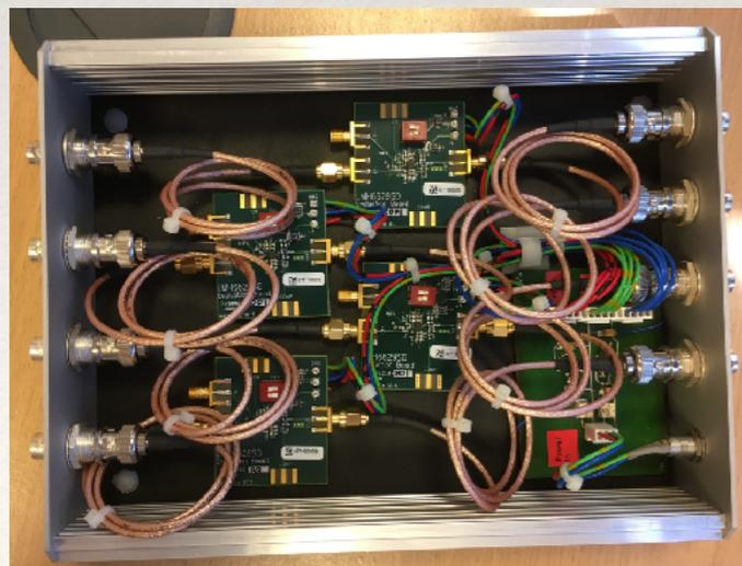
Fig.3. Signal amplifier assembly.
