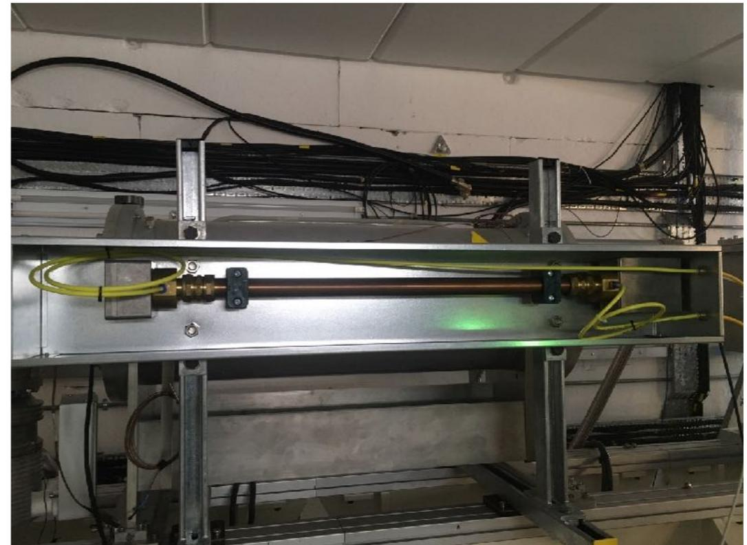
Fig. 2. Test demo-BLMs on FETS beam dump.
