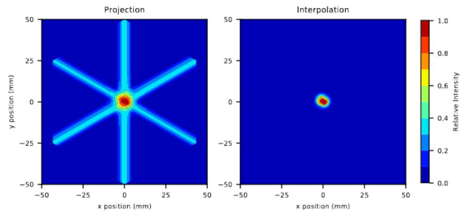
Figure 3.19: Reconstruction of  $10 \times 10 \text{ mm}^2$  6 MV X-ray field.
