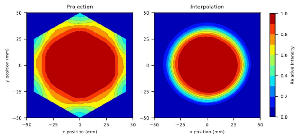
Figure 3.20: Reconstruction of  $30 \times 30 \text{ mm}^2$  6 MV X-ray field.
