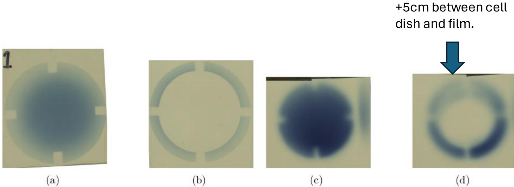
Figure 13: Film scans taken at the MC40 cyclotron facility. (a) film is inserted into cell dish holder without cell dish in place, (b) film is inserted into cell dish holder with cell dish in place, (c) set up as in Figure 12 without cell dish, (d) set up as in Figure 12 with cell dish.
